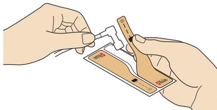
Peel new tape from backing and attach to sensor
